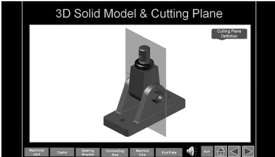
**Figure 4.** Shows a 3 D solid model of the machinist's jack and cutting plane
