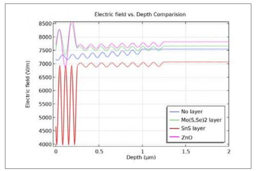
Figure 5: Electric field penetration based on the penetration of the electromagnetic radiation
