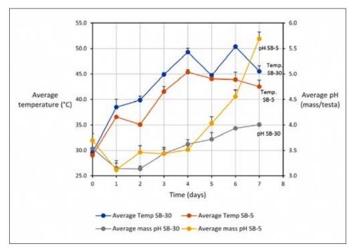
**Figure 2:** Comparison of average temperature and pH (mass) readings as fermentation progressed for SB-5 and SB-30 cacao fermentation prototypes.
