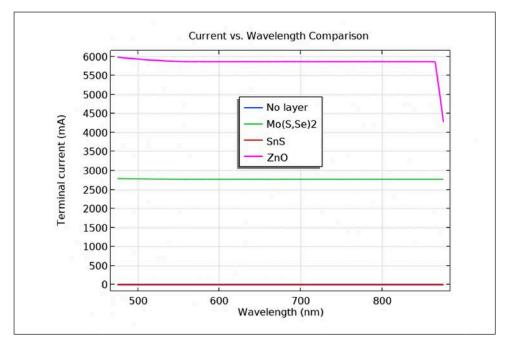
Figure 4: Current-Wavelength graph comparison. Note that the blue line is overlaid by the red line
