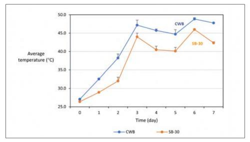
**Figure 3:** Comparison of average temperature trends as time progressed during cacao fermentation in Commercial Wooden Box (CWB) and SB-30 prototype.
